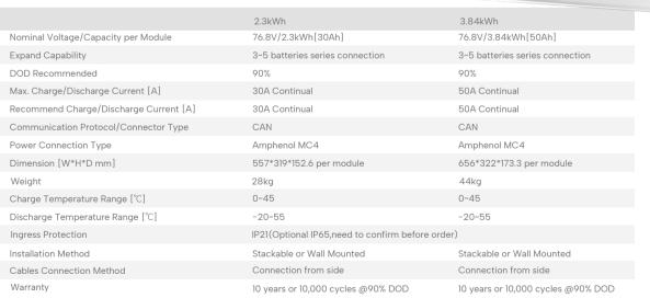
\*Battery System Configuration Options[2.3kWh]: 230V/6.9kWh, 307V/9.2kWh, 384V/11.5kWh,
